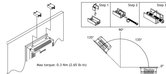
3. The PWS must be installed within an angle of 0° to 135° as shown above.
